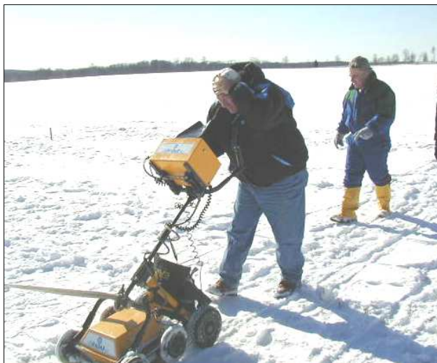
Surface-penetrating radar equipment can even be used when the ground is frozen.
